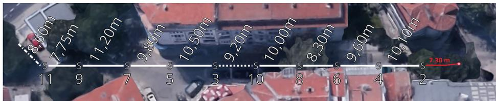
(b) Aerial photograph of the experimental setup showing the distance between each sensor (marked by white S) and the fire hydrant (red point on the rightmost side).
